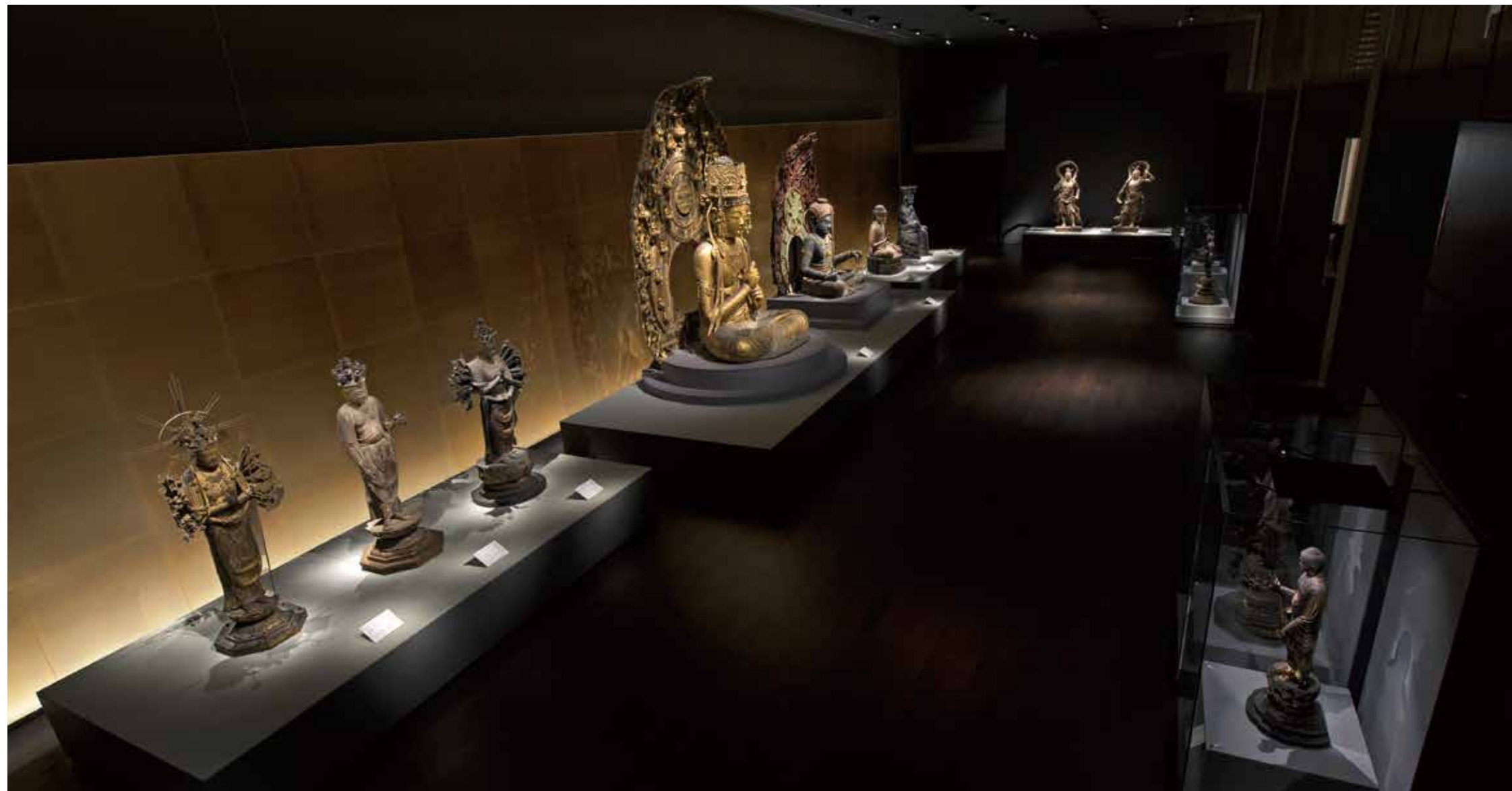
Overview of 1st floor sculpture gallery: Wall lighting from the floor and ceiling cascades over the sulfur oxidized brass finished wall behind the Buddhist sculptures
